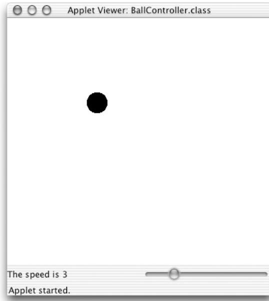
Figure 10.14: JSlider with JLabel in JPanel.
