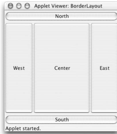
Figure 10.3: Layout of a window using BorderLayout layout manager.
