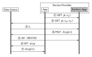
Figure 7: Protocol for the PMSys averaging function in a source-based monitoring architecture.
