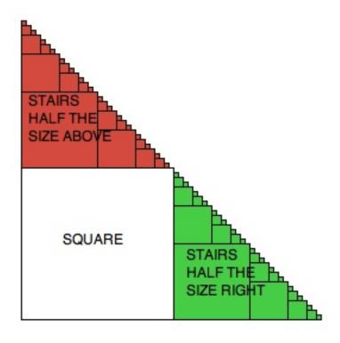
Stairs are specified by the x, y coordinates of the bottom left corner of the stairs and the length l of a size of the square in the lower left hand corner.
