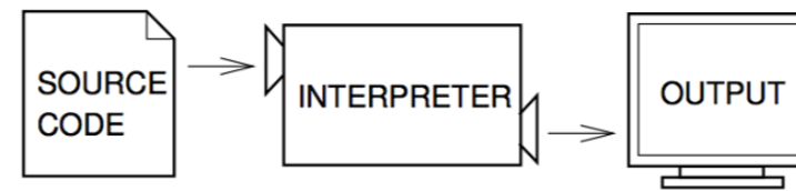
Figure 1.1: An interpreter processes the program a little at a time, alternately reading lines and performing computations.
