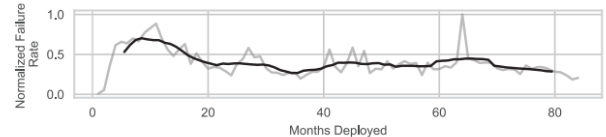
Fig. 2. Moving average (black) of raw (gray) normalized failure rates vs. DDR4 DIMMs’ deployment time in production. Failure rates tend to stay constant over a 7-year period.
