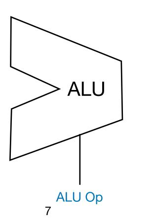
Wire set to "add" encoding by decoder!
