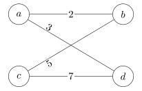
Apply Hungarian algorithm to find the min-cost perfect matching in G. First initialize the matching and prices, then make updates by searching for a good path (an alternating tight path between unmatched nodes). If no good path is found, update the prices on a good set. The final matching should have cost 8. Use the space below to record intermediate steps in the algorithm.
