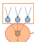
error for node is  $\sim w_i * \text{error}$
