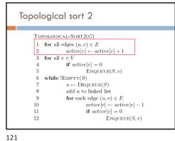
Topological sort 2 Topological-Sort2(G)1 for all edges  $(u, v) \in E$  $active[v] \leftarrow active[v] + 1$ 3 for all  $v \in V$ if active[v] = 0Enqueue(S, v)6 while !Empty(S)  $u \leftarrow \text{Dequeue}(S)$ add u to linked list  $\textbf{for each edge}\ (u,v) \in E$  $active[v] \leftarrow active[v] - 1$  **if** active[v] = 011 12 Enqueue(S, v)
