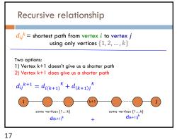
Recursive relationship  $d_{ij}^{k}$  = shortest path from vertex i to vertex jusing only vertices  $\{1, 2, \dots, k\}$ Two options: 1) Vertex k+1 doesn't give us a shorter path 2) Vertex k+1 does give us a shorter path  $d_{ii}^{k+1} = ?$ How do we combine these two options?
